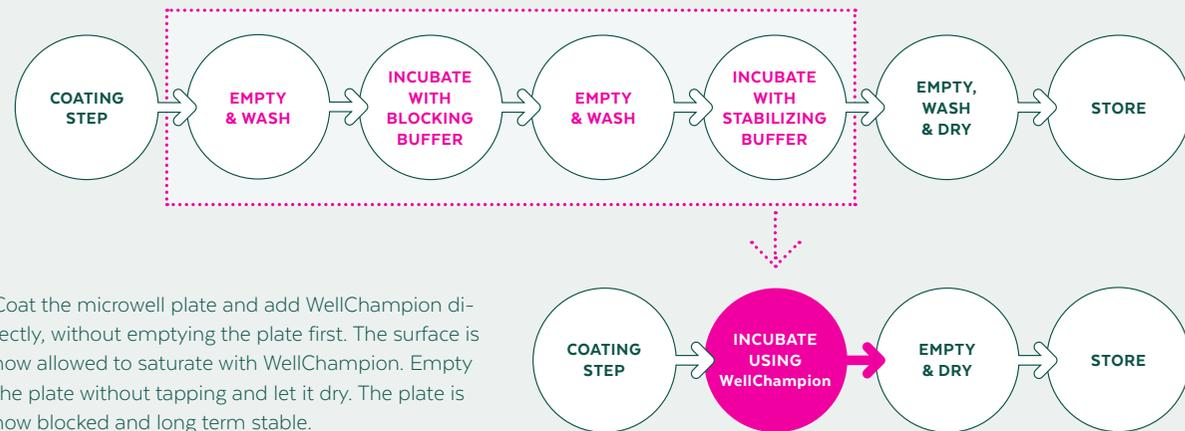
Coat the microwell plate and add WellChampion directly, without emptying the plate first. The surface is now allowed to saturate with WellChampion. Empty the plate without tapping and let it dry. The plate is now blocked and long term stable.
